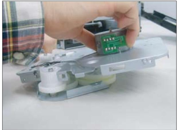
3. Remove 2 screws. Release the step motor.
