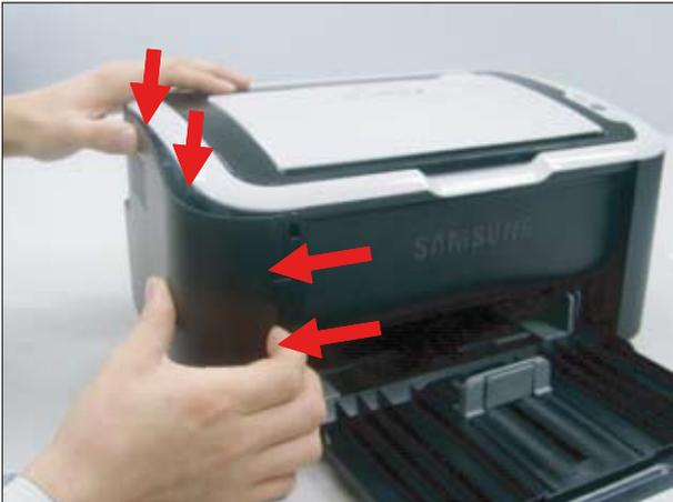
2. Take off the right cover by removing hooks from its edge.
